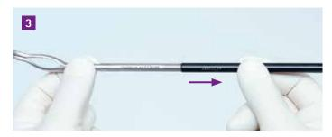
**Disassemble shaft I**Hold the jaw insert at the tip and remove the outer insulation
