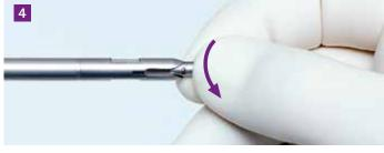
Disassemble shaft II
